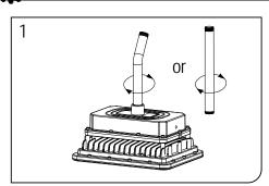
1. Take the fixture and pole accessory out from cartoon box, tighten pole as Fig.1. (Linear pole)
