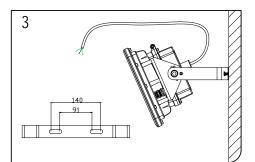
3. Drill 2x hole as Fig.2, the distance can be 91~140mm, fixing Ø10 expansion screws and bracket on wall.
