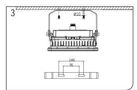
3. Drill 2x hole as Fig.2, the distance can be 91~140mm, fixing Ø10 expansion screws and bracket on ceiling.
