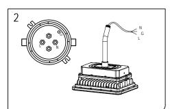
2. Connect the AC cable to installation box, Black cable joins to L, white cable joins to N, green cable joins to grounding.
