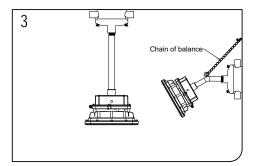
3. Install the installation box to the wall or ceiling as FIg.2. Tighten the pole to the box, and adjust the chain of balance.
