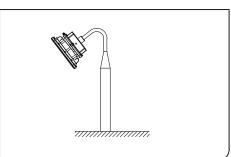
Install the fixture to the pole after cable connecting.
